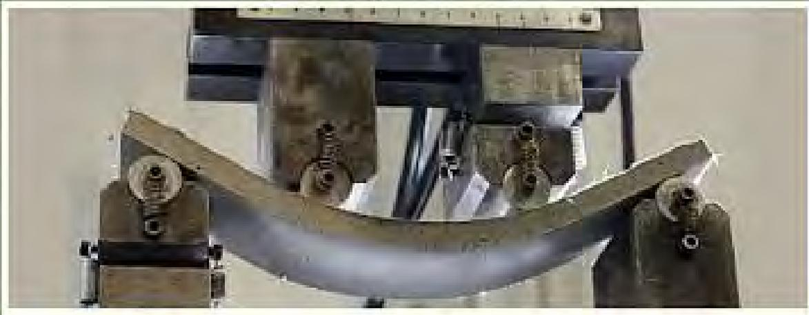
**"Self-healing Concrete: By devising concrete that controls the way it cracks under stress, the concrete can withstand tensile strain hundreds of times more than ordinary concrete. Beyond its remarkable flexibility, this concrete can then heal itself, as well."**
