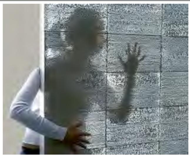
**"The translucent concrete, or LitraCon, is the invention of Hungarian architect Aron Loconcz, which deals with concrete plus fiber optics. The fibers are mixed into the concrete, forming a series of "channels" glass, which makes possible the passage of light. This way you can create this effect of translucency on an object far seen only as a solid object and opaque."**
